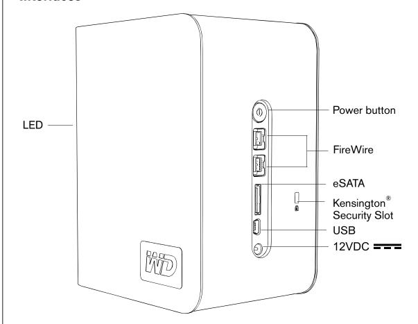
**FireWire** – This device is equipped with two FireWire 800 interfaces. FireWire 800 has a maximum data transfer rate of 800 Mb/s and is backward-compatible with FireWire 400 using a special adapter such as the FireWire 800 to 400 cable included in this kit. Connection to a FireWire 400 device transfers data at FireWire 400 speed (up to 400 Mb/s).
